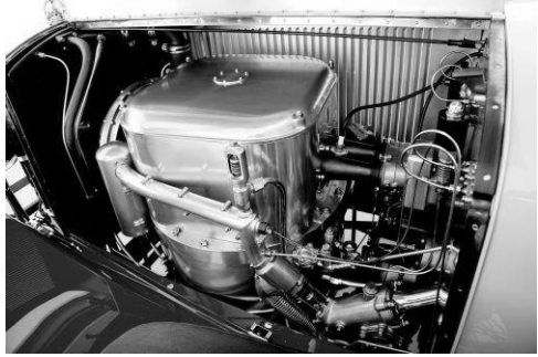
The Doble Steam boiler of 1925.
