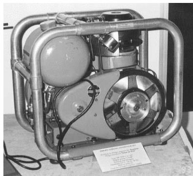
A Stirling engine portable generator that was manufactured in the 1960s
