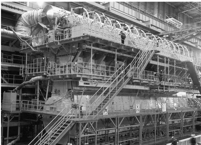
The first 14-cylinder Wärtsilä RT-flex96C marine engine has a maximum continuous power output of 80,080 kW (108,920 bhp) at 102 rpm. Measuring 27.3 m long and 13.5 m high, it has an overall weight of 2300 tonnes.
